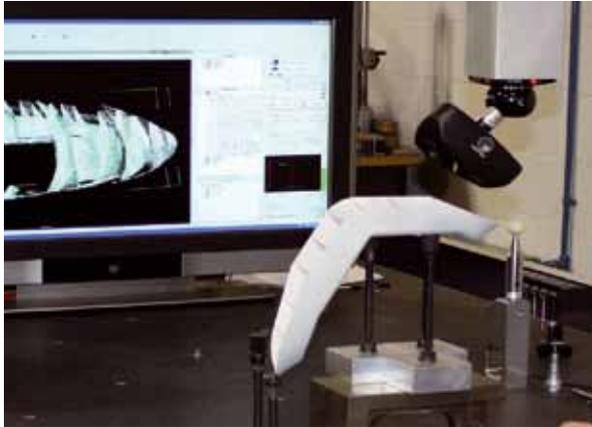
*Nikon Metrology's Cross Scanner acquired the entire geometry of the wing tip light housing.*
